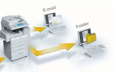
Via the LAN fax function, you can send fax messages directly from your own PC. This saves time and results in better output quality at the receiving end. To reduce the distribution of printed faxes, faxes can also be forwarded by e-mail.
